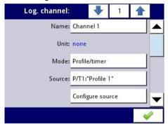
Fig. 7.61. View of the input channel configuration in Profile/timer mode
