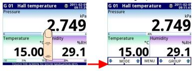
Fig. 6.6. Main window of the device – displaying the Navigation bar
