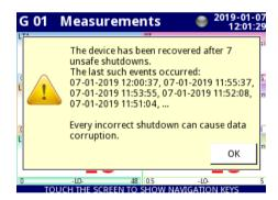
Fig. 6.3. The view of the screen with a message about 7 unsafe shutdowns
