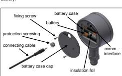
Fig. 3 Battery case and communication interface
