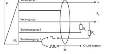
3-wire system (IO-Link / SIO with analog output)
