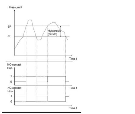
Fig. 4 Switching and resetting behavior for hysteresis function in pressure-time graph
