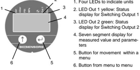
Fig. 3 Control pad for device with 2 switching outputs
