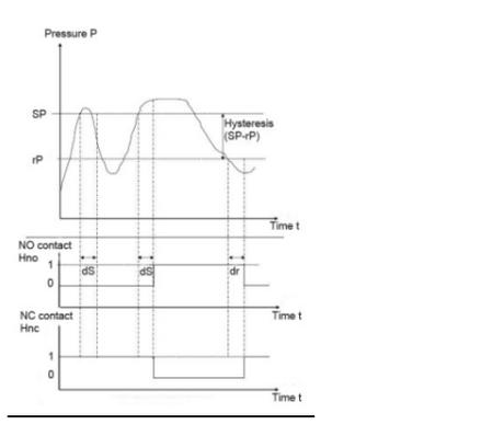
Fig. 5 Switching and resetting delay for hysteresis function in pressure-time graph
