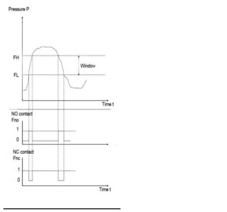
Fig. 6 Switching and resetting behavior for window function in pressure-time graph
