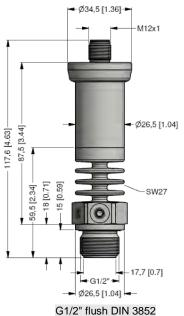
G1/2" flush DIN 3852 with cooling element 200 °C
