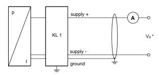
The ground wires of all components have to be connected!
